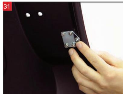
31 Install a wave washer onto the 20° bracket.
