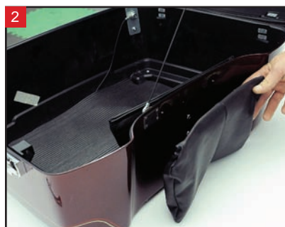
2 Remove the lower passenger backrest.
