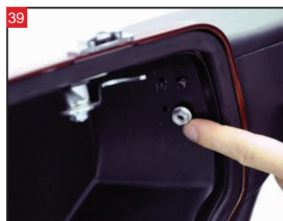
39 Install the backrest mounting hardware.
