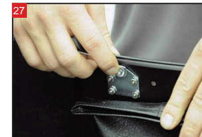
Install the brace arm onto the 5° bracket.
