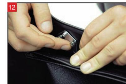
12 Install the nuts onto the mounting bolts.
