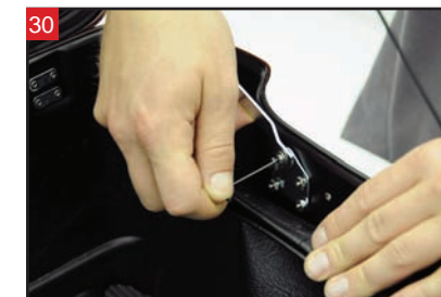
Tighten the brace mounting hardware.
