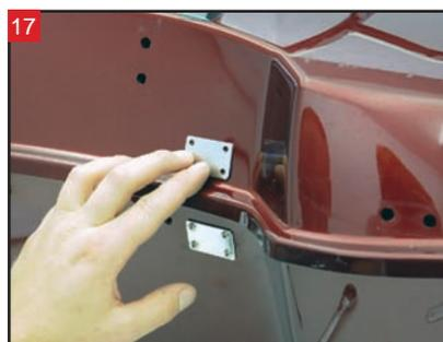
Position the upper backing plate directly above the lower.
