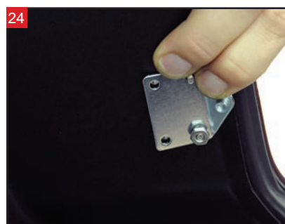
Install the nuts on the bolts.
