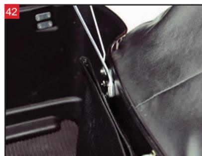
42 Tighten the lower backrest mounting hardware.
