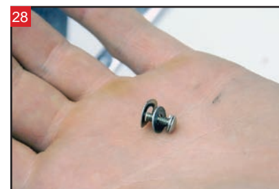
Install a lock washer, regular washer, and wave washer on the brace bolt.
