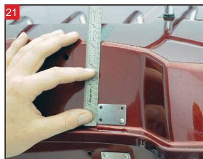
Measure the mounting bracket to make sure it's level.
