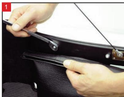
1 Loosen the lower passenger backrest mounting hardware.
