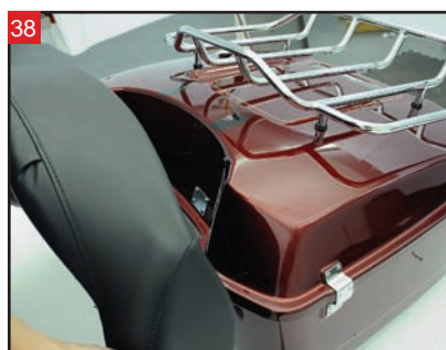
38 Install the upper passenger backrest.
