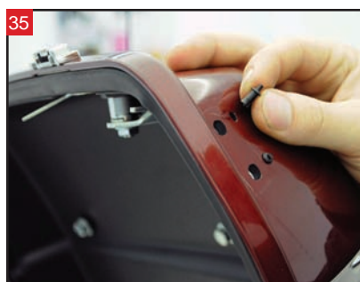
35 With the pins pushed out, remove the retainers.
