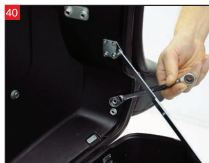
40 Tighten the backrest mounting hardware.
