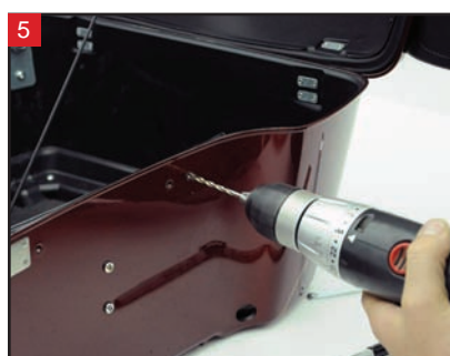
5 Drill the marked hole in the Tour-Pak.
