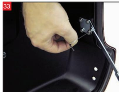
33 Tighten the mounting hardware.
