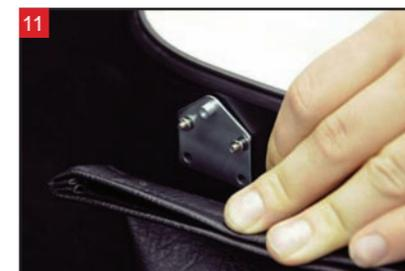
11 Install the mounting bolts and lock washers.
