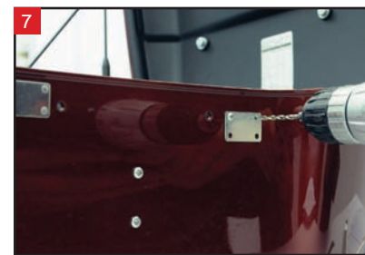
7 Use the mounting plate as a drill guide for the rest of the holes.
