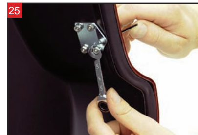
Tighten the mounting hardware.
