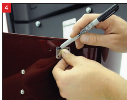
4 Mark the location of the first hole in the backing plate.
