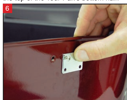
6 Place the backing plate up to the Tour-Pak and install a bolt through the first hole.
