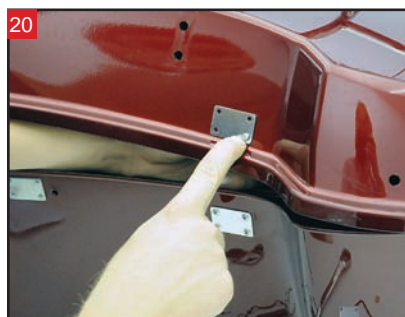
Install one of the mounting bolts.
