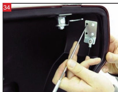
34 Use a pick to push out the lock pins in the stock tether mount.
