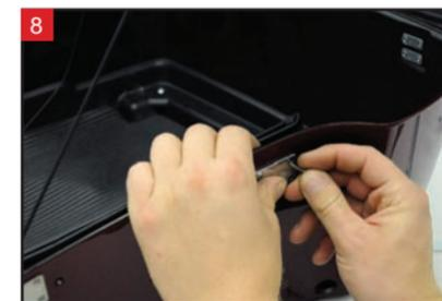
8 Remove the bolts holding the backing plate in position.
