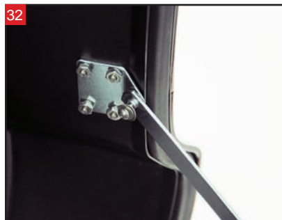
32 Install the mounting bolt (with the three washers) into the bracket.
