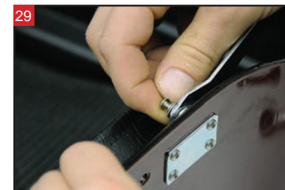
Install the brace bolt through the brace, and into the mounting bracket.
