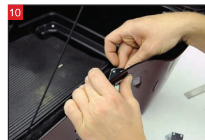
10 Install the backing plate and 5° mounting bracket.
