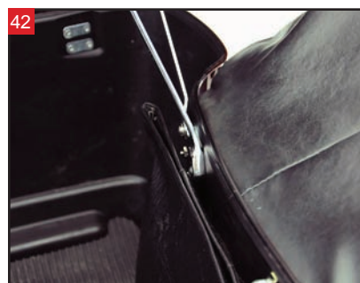
42 Tighten the lower backrest mounting hardware.
