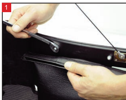
1 Loosen the lower passenger backrest mounting hardware.
