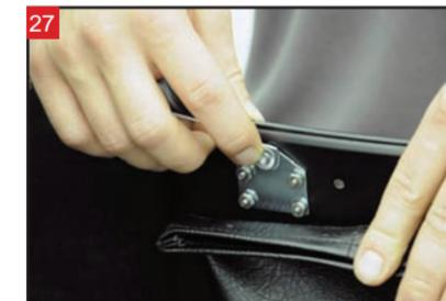
Install the brace arm onto the 5° bracket.
