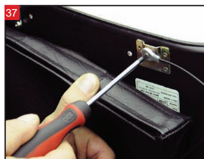
37 Unscrew the stock lower mounting bracket and remove the tether.
