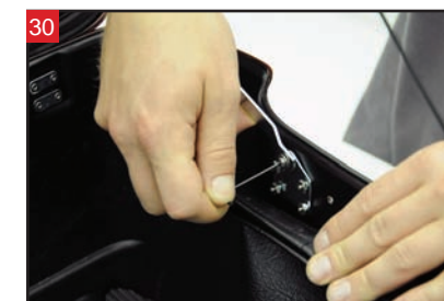
Tighten the brace mounting hardware.
