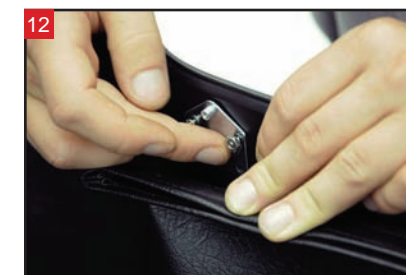
12 Install the nuts onto the mounting bolts.
