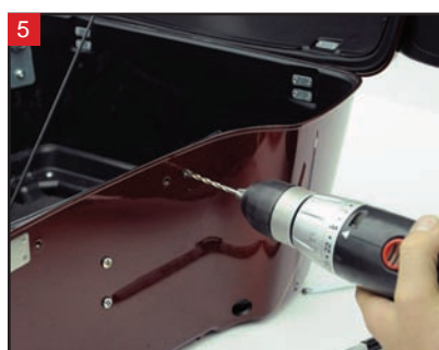
5 Drill the marked hole in the Tour-Pak.
