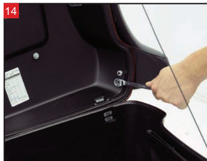
Remove the left-side upper passenger backrest mounting hardware.
