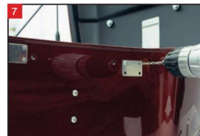
7 Use the mounting plate as a drill guide for the rest of the holes.
