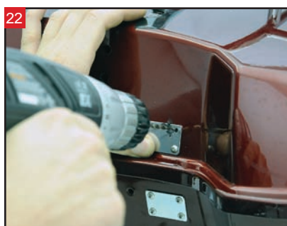
Drill the rest of the holes using the backing plate as a guide.
