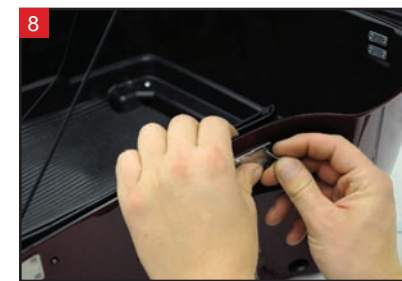
8 Remove the bolts holding the backing plate in position.
