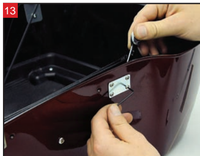
Tighten the mounting hardware.
