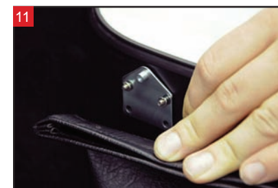
11 Install the mounting bolts and lock washers.
