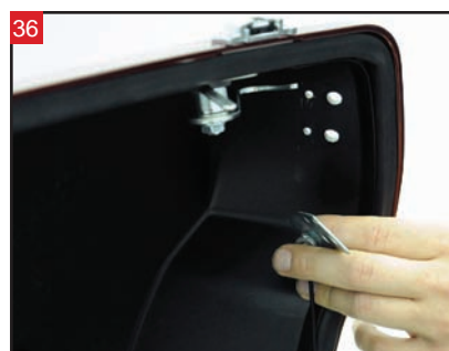
36 Remove the upper stock mounting bracket.
