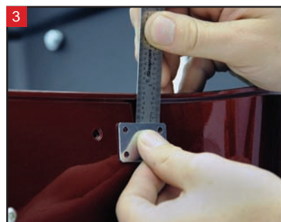
3 Place the backing plate on the opposite side of the stock tether bracket, 3/4" from the top of the Tour-Pak's bottom half.
