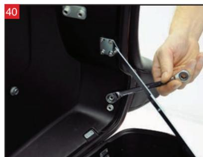
40 Tighten the backrest mounting hardware.
