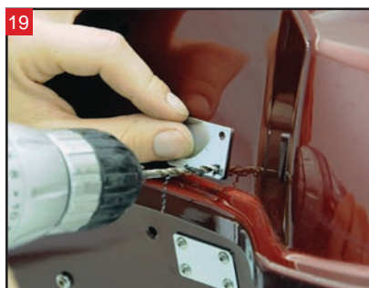
Drill the first hole for the upper mount.
