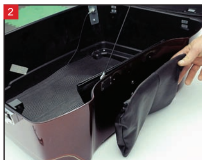
2 Remove the lower passenger backrest.
