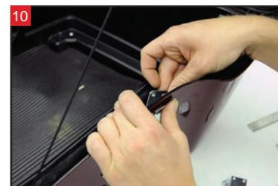
10 Install the backing plate and 5° mounting bracket.
