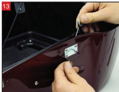
Tighten the mounting hardware.
