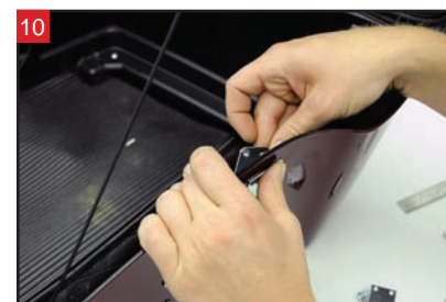
10 Install the backing plate and 5° mounting bracket.
