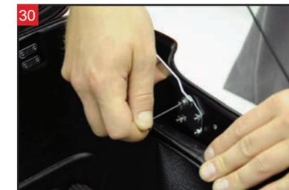
Tighten the brace mounting hardware.
