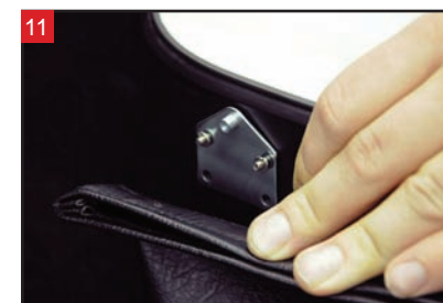
11 Install the mounting bolts and lock washers.
